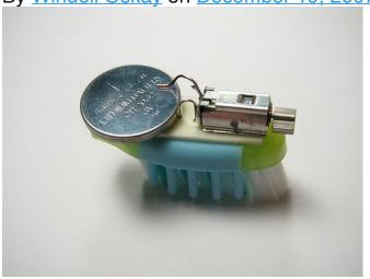
The BristleBot is a simple and tiny robot. One toothbrush, a battery, and a pager motor.
