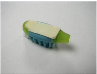
The last substantial ingredient is some foam tape. Apply a small piece to the top of the toothbrush robotic platform, which will be used to hold the motor in place.
