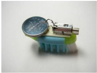
A better method is to bend one of the leads down flush with the foam tape, so that you can \*stick\* the battery to the foam tape as well and still make an electrical connection. The other lead contacts the other side of the battery, and the motor can run,
